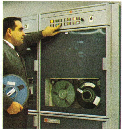
Input . Just as a bookkeeper reads a check, above, to put information into his head, a tape unit, below, reads magnetic tape to put information into a computer. The bottom photo shows the part of the machine that reads the tape.
